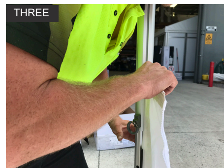
Insert the top section of the of the Wall Strip Keda into the tracking of the Upper Leg of Canopy.
