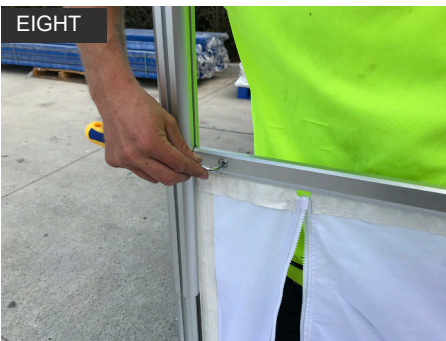
Using the supplied tool, tighten the bolt lightly. Repeat on other side. Adjust the Half Wall Bar as need to be level and in desired position, tighten bolts to secure.
