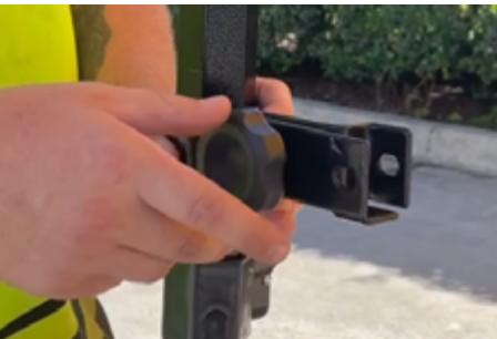
1. Attach half wall display connector to tent leg. Repeat on other side.
