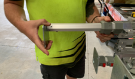
1. On a bench or on the ground lay tent on side, extend inner leg of tent.
