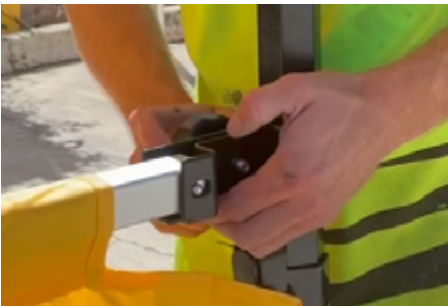
3. Insert half wall display bar into connector and tighten the connector. Repeat.
