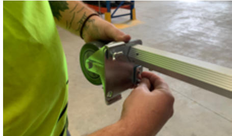
3. Tighten the wing nuts on the left/right until finger tight. Repeat until all wheels are fitted to tent legs.
